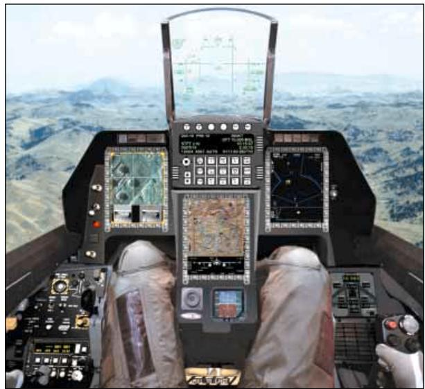
**Green Hills RTOSes support processing for the panel displays and head-up display of the F-16E/F, Block 60.**
