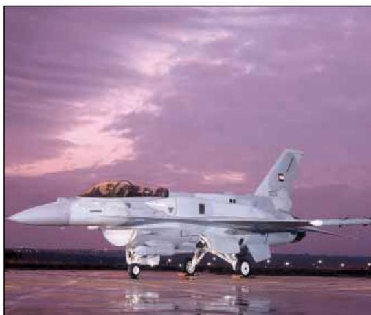
**The F-16E/F, Block 60, will feature new sensors, displays and high-speed fiber optic links.**
