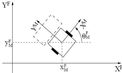
Fig. 5. Mobile ( $M$ ) and Fixed ( $F$ ) coordinate systems.
