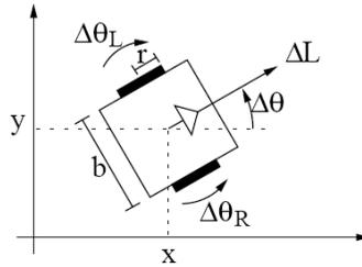
Fig. 2. Variables of the kinematic model.
