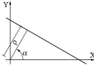
Fig. 4. Line parameters:  $\rho$  and  $\alpha$ .
