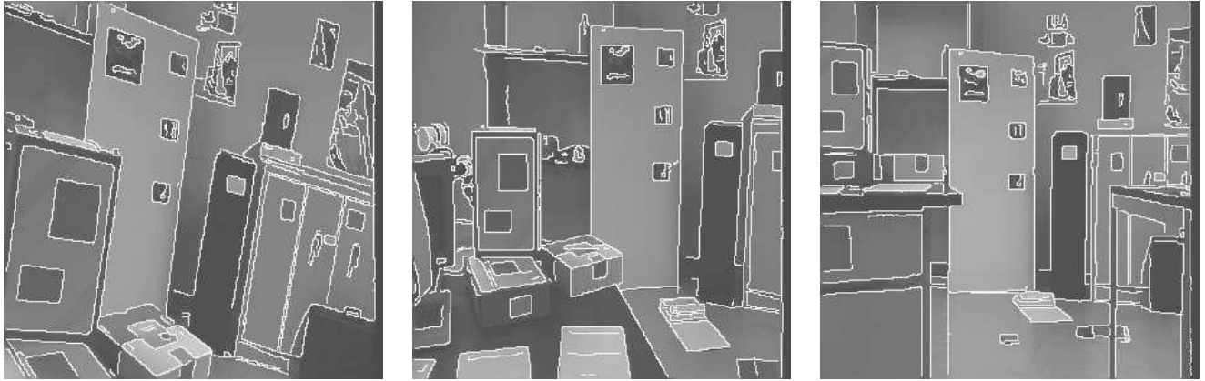
Figure 19: The triplet of images of the indoor scene, with edge chains superimposed.
