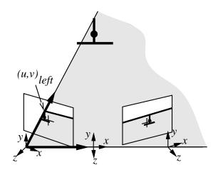
**Epipolar plane:** defined by the line joining the focal points of the stereo system and the ray from the left focal point to the image feature of interest.
