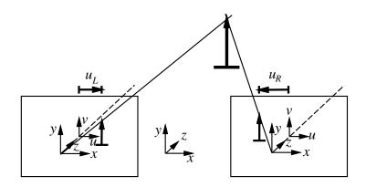
Consider this simple binocular configuration. In this geometry, the stereo system encodes depth entirely in terms of disparity. Under these conditions
