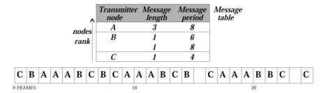
**Fig. 1.** Example of implicit contention using EDF.
