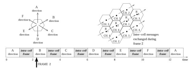
Fig. 2. Example of intercell communication mechanism using TDM.
