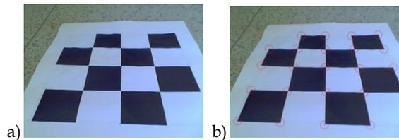
Fig. 7. Calibration pattern.
